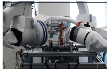
Figure 1: Photograph of cadaveric wrist simulator and bi-plane fluoroscopy system imaging a wrist specimen undergoing dynamic wrist flexion
