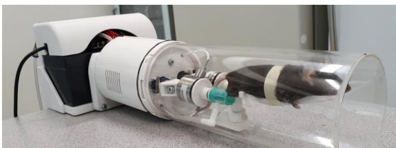
Figure 1: The device for image-guided mechanical evaluation of the murine knee.
