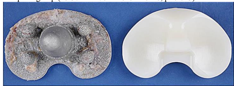
Figure 1: Retrieved tibial base plated covered or with traces of fibrous tissue with insufficient osseointegration
